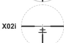
X02i Cross shaped reticle with illuminated dot and a scale allowing distance measurement to an object with known sizes and windage/elevation scale 9/12x.
