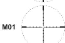
M01 Mil-Dot reticle, works correctly if magnification is set to 9/12x.
